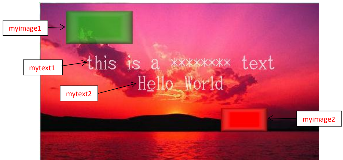
Fig 2.16 Screen shot of what you will see on the TFT module when example code in Fig 2.17 is uploaded
