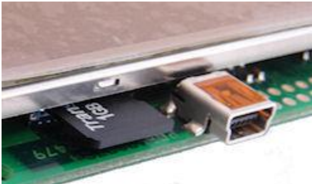
Fig. 8.1 Image of a 1GB micro SD card inserted into CN9 of the TFT module
