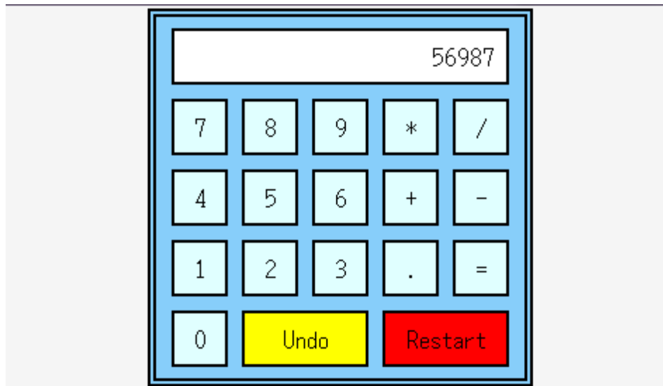
Fig. 3.67 Screen shot to demonstrate what will be observed on the display when the code in Fig 3.68 is uploaded onto the TFT module
