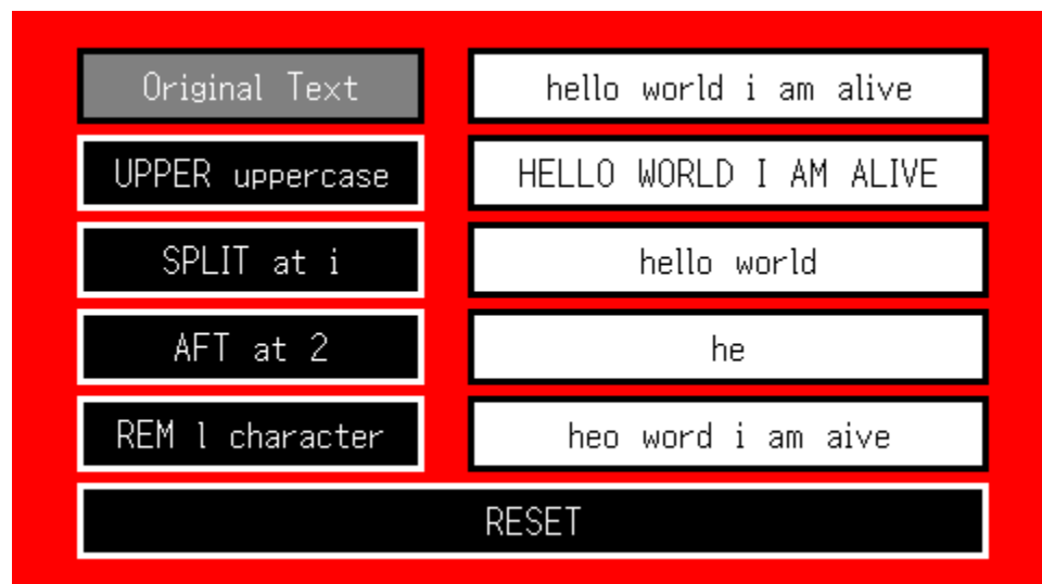
Fig. 3.71 Screen shot demonstrating the changes that would occur when the text handling methods using the CALC command is applied
