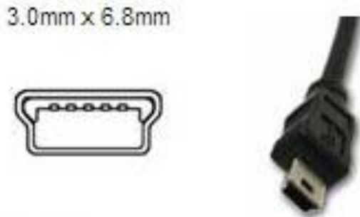
Fig. 8.14 Image of the standard mini-B USB cable connector
